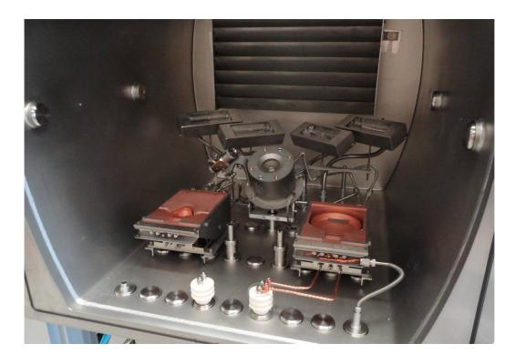
Example showing four heater modules mounted at the rear of the chamber Heater modules come complete with lamps, glass, feedthrough and connectors.
