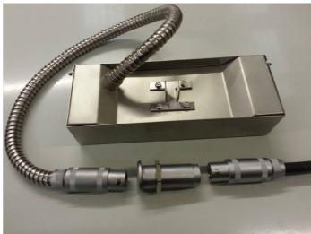
The body of the unit is made of stainless steel with a molybdenum reflector and the quartz halogen lamps are protected from coating deposits by a sheet of high temperature furnace glass. The cover is easily removed to enable replacement of the lamps or glass.
